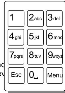
The method of entering the characters is similar to the method employed on mobile telephones. The number buttons provide both their appropriate number and several letters of the alphabet. An example of the keypad is shown opposite.
