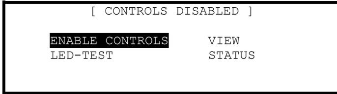
To enable the controls, ensure the "Enable Controls" option is highlighted and then press the ✓ button. The display then requests entry of the Level 2 or 3 passwords as follows:
