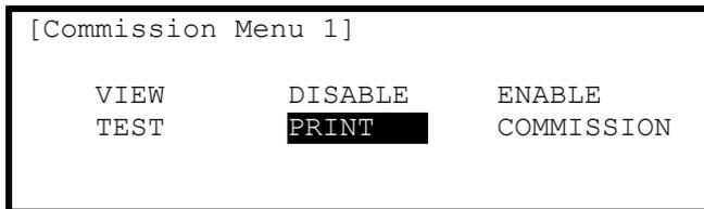
When a menu is displayed, use the  $\leftarrow\uparrow\downarrow\rightarrow$  buttons to highlight the required menu option and then press the  $\checkmark$  button to select it.
