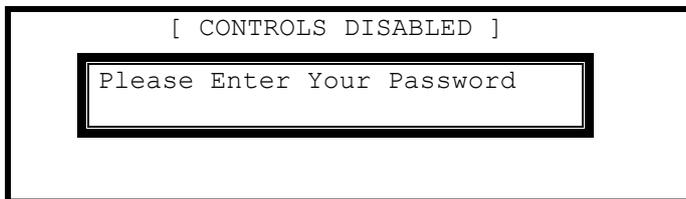
Enter the password using the number buttons and then press the ✓ button. As each number is entered, an asterisk (\*) is shown on the display. For example:
